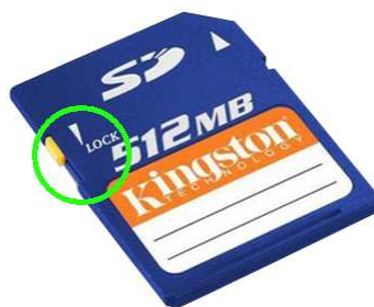
Figure 9 : SDCard write protect switch
